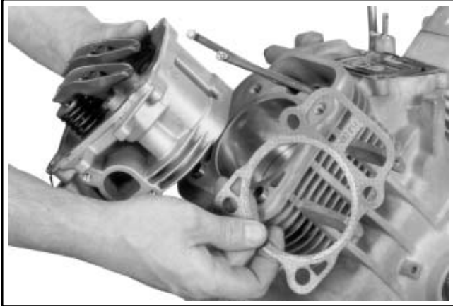
Figure 11-40. Always Use New Head Gaskets.
